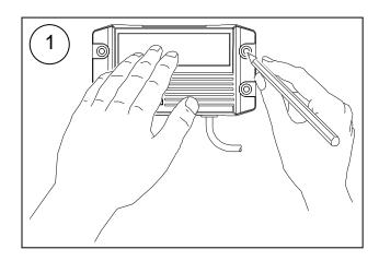
Mark the position of the four mounting spots. Remove the charger and drill the mounting holes. Fix the charger to the wall using corrosion resistant 4.8mm (3/16") dia. or M5 (#10) bolts, backed by a flat washer, and secured to the mounting surface with a split-ring lock washer.
