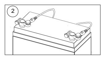
When connecting the battery, the ungrounded terminal must be connected first. Connect the RED charger output to the POSITIVE (POS, P, +) battery post; connect the BLACK charger output to the NEGATIVE (NEG, N, –) battery post.
