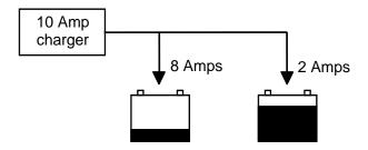
If the two batteries have drained equally, the charger will send the same amount of power to each battery.
